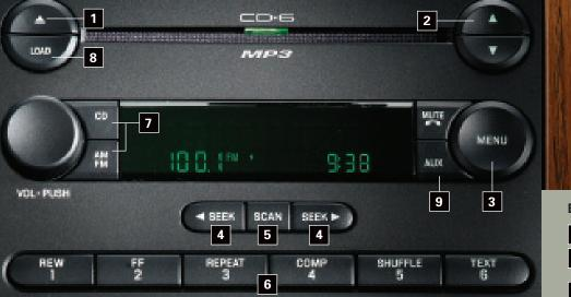
1 EJECTING CDS (CD EJECT): Press to eject a CD. For In death CDC (1975) (if equipped), press and hold to auto-eject all CDs present in the system.
